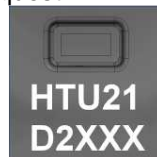
Laser marking on HTU21D sensor
