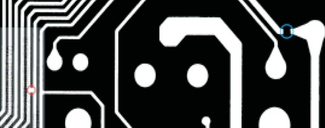
PCB断路检测 PCB open circuit detection
